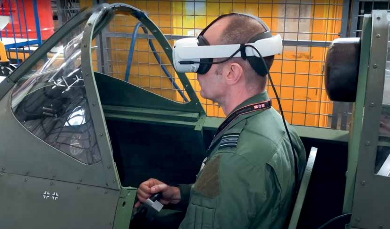
↑ BBMF fighter pilot Sqn Ldr Mark 'Disco' Discombe flying the Spitfire virtual reality "Flying Training Device". Disco has been instrumental in developing the "simulator" as a BBMF fighter pilot emergencies training device. (Photo: BBMF)
