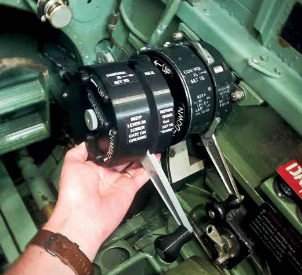
An AuthentiKit 3D-printed Spitfire "Chassis" undercarriage lever alongside the real thing in one of the BBMF's Spitfire cockpits. (Photo: BBMF)
